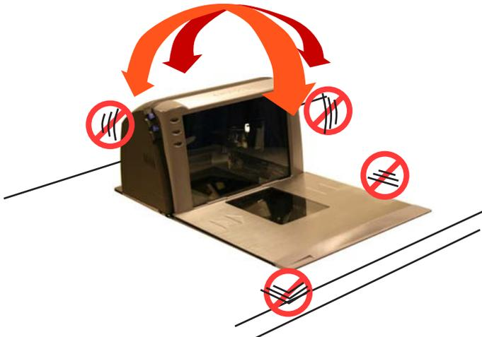
The product must be mounted in the counter in a stable position. Check to ensure that it does not rock or “teeter” from side-to-side or corner-to-corner on any axis.
