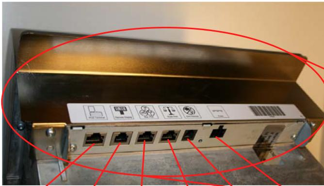
POS I/F    Remote Scale Display    Aux. Port    Scale Host Port    EAS Interlock    Power
