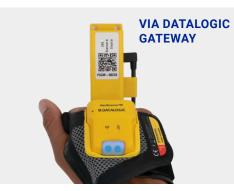
Scan the Pairing Barcode on the top of the Datalogic Gateway.
