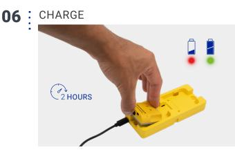
The pins face down. Insert the HandScanner in the Datalogic Charging Station.
