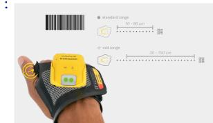
Press the textile trigger. Aim at the barcode and scan.
