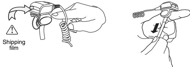
1. Remove the shipping film from the ring scanner window.
