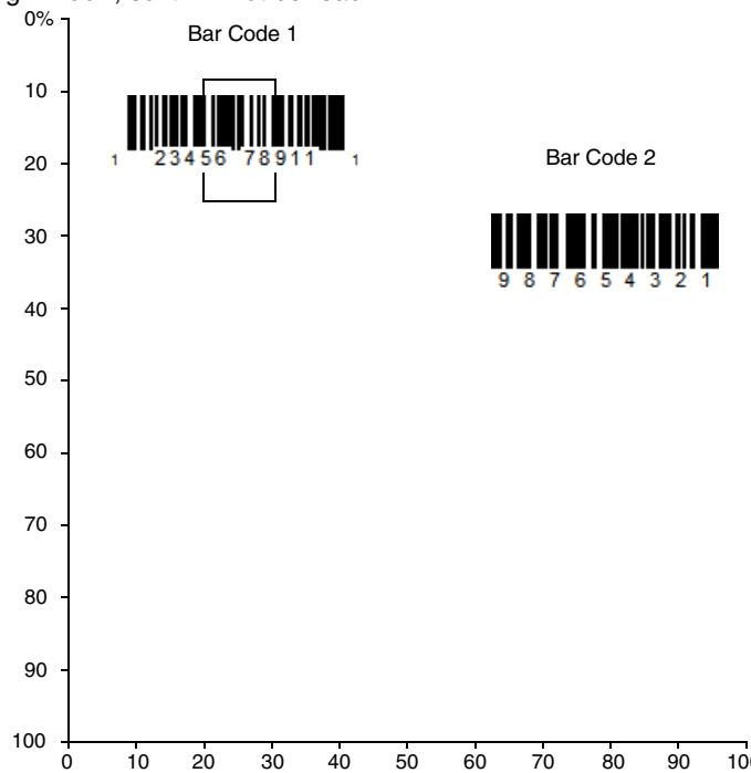
*Note: A bar code needs only to be touched by the centering window in order to be read. It does not need to pass completely through the centering window.*
