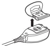
3. Place the trigger on the ring scanner and screw in the 4 screws to secure the new trigger.
