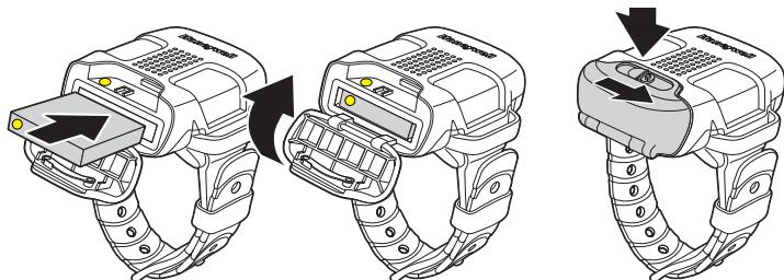
The 3.7V, 750mAh lithium ion battery in the Bluetooth module is designed to power the Bluetooth module for 8 hours and remain in standby for approximately 24 hours. Batteries are not fully charged when shipped. The battery should be charged for a minimum of 4 hours before initial use to ensure optimal performance.
