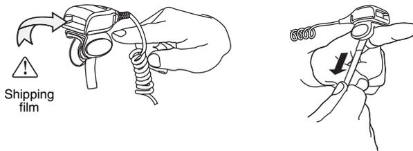
1. Remove the shipping film from the ring scanner window.
