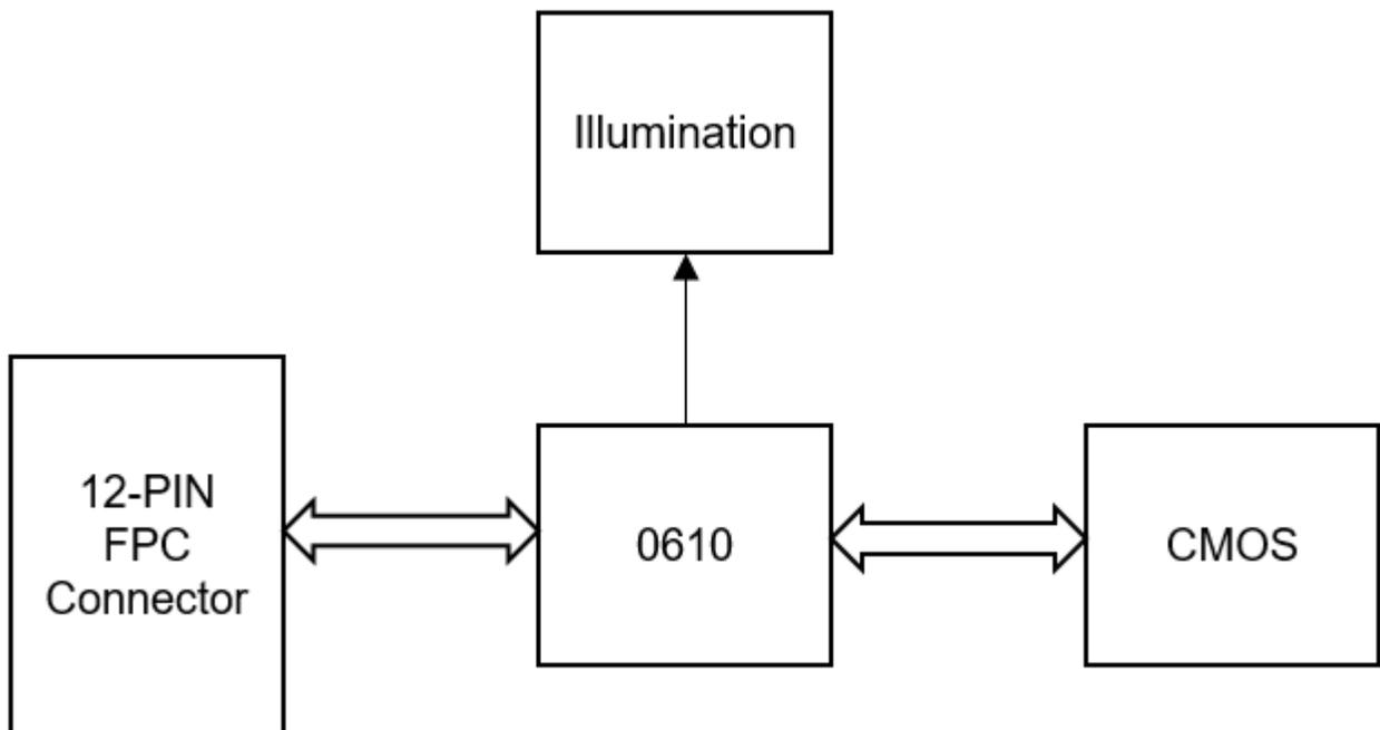
The engine connected with the host via the 12-pin FPC cable. For more details about the 12-pin FPC cable, please see **12-pin FPC** in Chapter 4.
