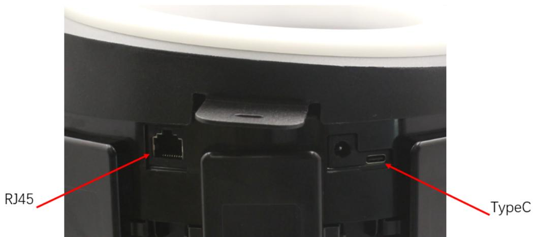
The device's serial port signals adopt the RS232 protocol, located at pin 4 and pin 5 of the RJ45 interface. Pin 4 serves as the device's serial port transmission signal, while Pin 5 serves as the device's serial port reception signal.
