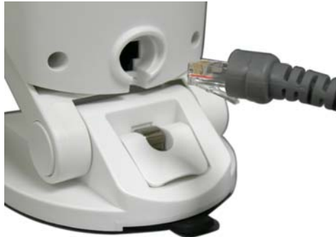
Figure 6: Interface cable connection
