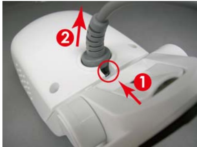
Figure 7: Replaceable interface cable
