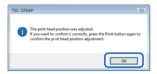
11. Click [Print] again to print a detailed head position adjustment pattern and check that the head positions have been adjusted correctly.
