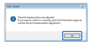
**16.** Click [Print] again to print a head position adjustment pattern and check that the head positions have been adjusted correctly.
