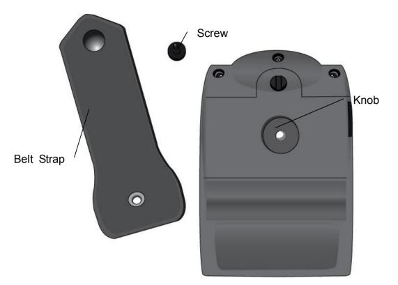
2. Attach the Belt Strap onto the Knob.
