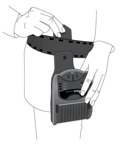
5. Pull down the top of the Belt Strap to fix onto the lock:
