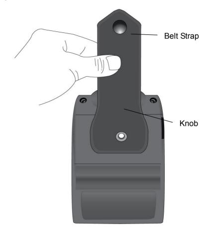
3. Insert the Screw onto the Knob, through the Belt Strap, and tighten clockwise until it is fully secured:
