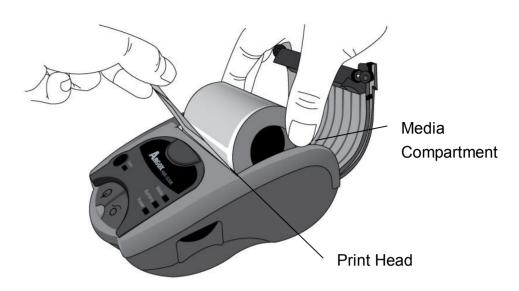
3. For media supply rolls with width less than 3 inches: Load media supply first, and then align media supply roll to the right end for correct detection of Media Sensor:
