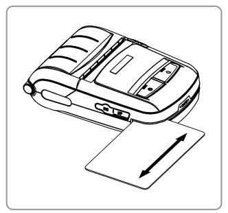
1) Insert the card as shown in the image and swipe in the direction of the arrow. (can be done in both directions)
