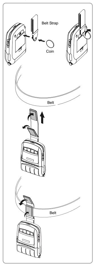
1) Insert the belt strap screw into the belt strap hole.
