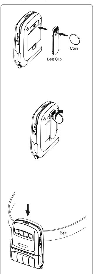
1) Insert the belt clip screw to the belt clip mounting hole.
