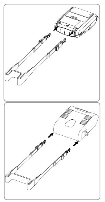
1) Connect the clips of the shoulder strap to the printer as shown in the figure on the left.
