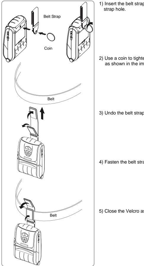
1) Insert the belt strap screw into the belt
