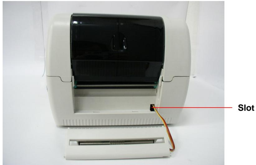
6. Lift up the lower inner cover to gently push strip panel into the two concaves of lower cover front side.
