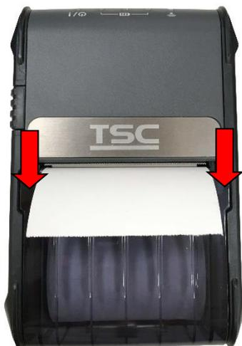
3. Press the media cover on both sides to close it and make sure the media cover have closed correctly.
