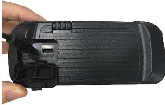
1. Open the interface cover and plug the power cord in to the power jack.
