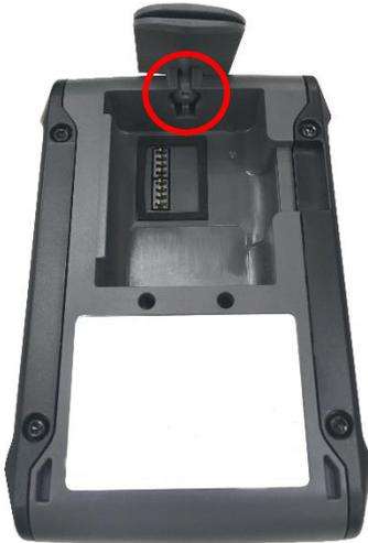
2. Press the ball on the belt clip to the hole as pictured.
