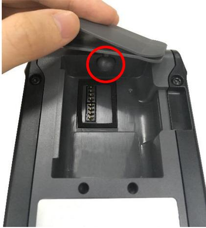
1. Remove the battery on the rear of the printer and lock the belt clip on the hole above the battery.
