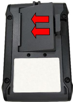
1. Insert the left side of battery to the slot on the rear of the printer.
