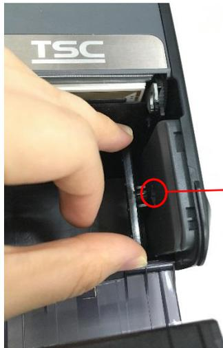
1. Open the printer top cover and install the media adapter in the media fixing hole as indicated.
