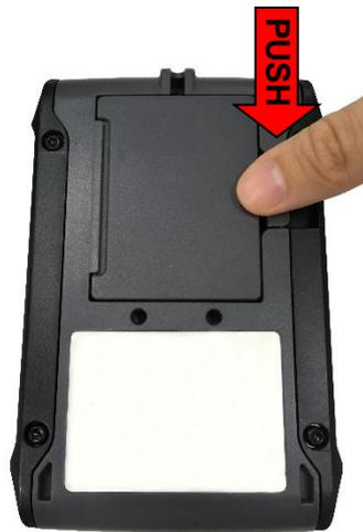
2. Push the right side of the battery clasp down and lock the battery.
