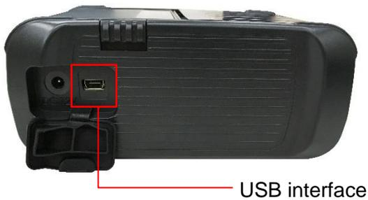
1. Open the interface cover and connect the printer to the computer with USB cable.
