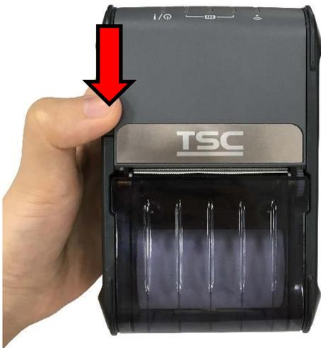
1. Open the printer media cover by pressing the media cover release button.
