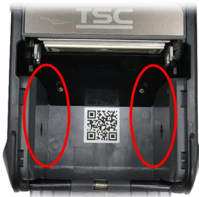
2. The media adapters are installed in the media fixing hole on both sides.
