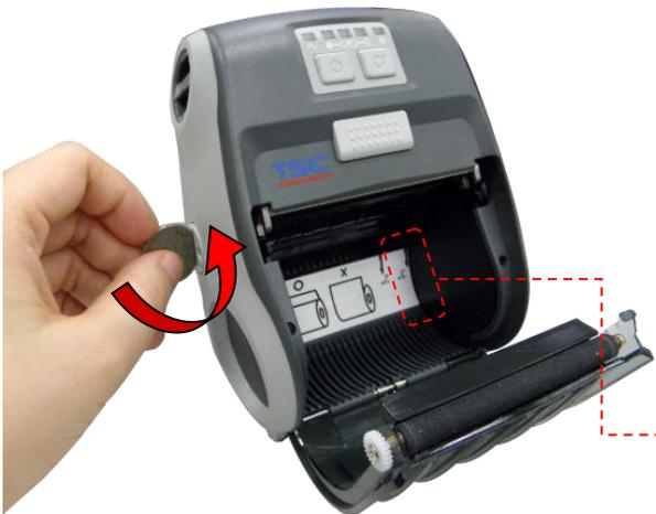
2. Use a coin to rotate the media holder adjustment knob, and the media holder should be placed at the correct place to fit the media roll.
