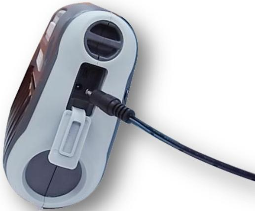
1. Open the interface cover and plug the power cord to the power jack.
