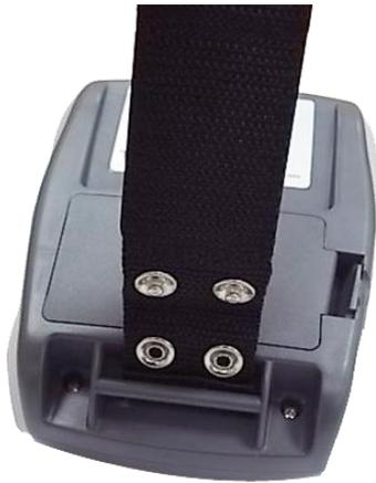
1. Refer to figure beside. Loop the belt clip through the slot below the battery.
