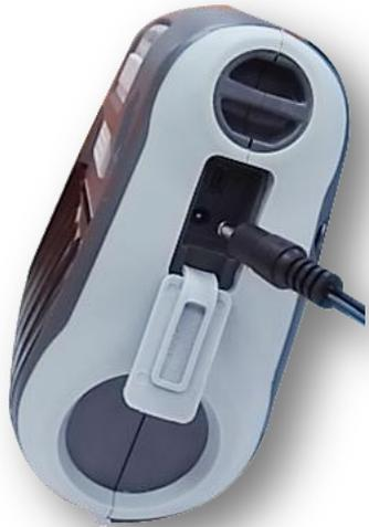
1. Open the interface cover and plug the power cord to the power jack.
