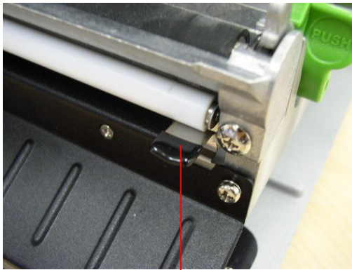
Peel-off roller release lever
