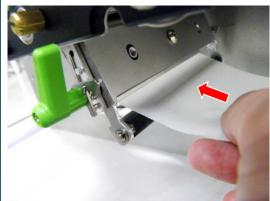
7. Press the middle of the peel-off roller to close the peel-off roller release lever.
