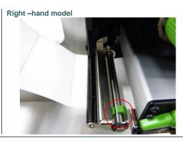
5. Adjust the front label guide (green) to fit the label width.
