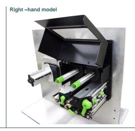
2. Push open the print head release lever and label guide bar release lever for loading media.
