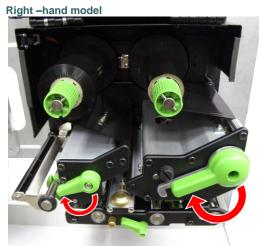
3. Pull the leading edge of the label forward through the media guide bar pass media sensor, and place the leading edge onto the platen roller.
