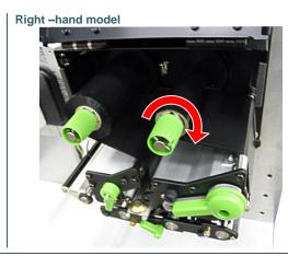
6. Close the print head mechanism by pushing the print head release lever.
