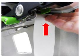
8. Close print head release lever and label guide bar release lever.
