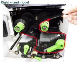
5. Wind the ribbon rewind spindle counterclockwise roughly 3~5 circles until ribbon is smooth, properly stretched and wrinkle-free.
