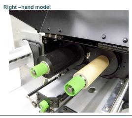
3. Push print head release lever to open print head mechanism.
