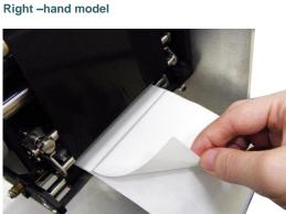
5. Open the peel-off roller release lever.
