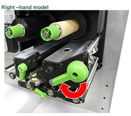
4. Thread ribbon above the ribbon guide bar and through ribbon sensor slot. (Please refer to "Loading path for ribbon" as following fig.)
