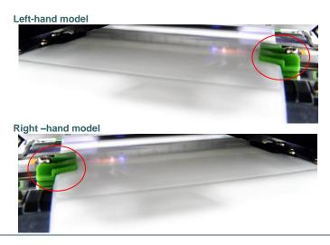
6. Move the media sensor by adjusting the media sensor position adjustment knob, make sure the gap or black mark sensor is at the location where media gap/black mark will pass through for sensing.
