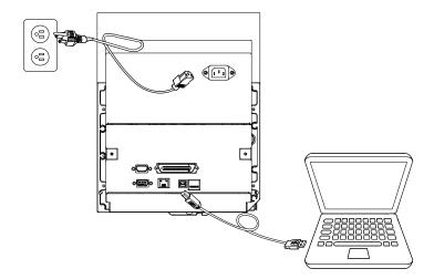
Note: Please switch OFF power switch prior to plug in the power cord to power jack.
