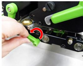
6. Feed the leading edge of liner through the peel-off roller.
