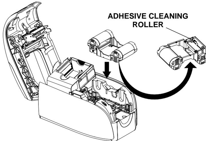
3. Insert the ribbon cartridge with the cleaning roller facing down, so the gears on the ends of the rollers fit into the appropriate slots.
