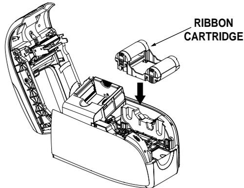
5. Insert the ribbon cartridge with the cleaning roller facing down, so the gears on the ends of the rollers fit into the appropriate slots.
