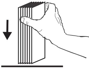
4. Holding the card deck by the sides, hold it vertically against a flat surface such as a desktop. If the deck is too thick for your hand to hold it comfortably, use about half a deck at a time.
