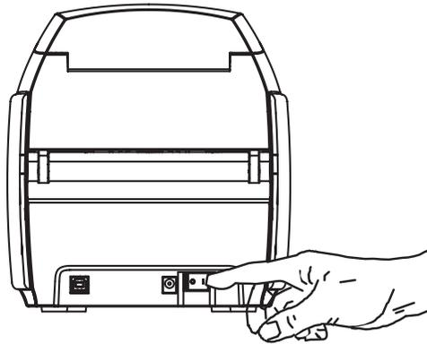
1. Place the printer power switch in the ON (|) position.
