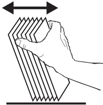
5. Push the stack back and forth to an angle of about 45° from vertical, so as to separate all of the cards.
