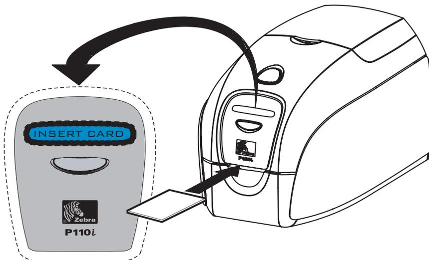
2. Insert a single card into the slot at the front of the printer, directly above the card output hopper. Do not feed more than one card at a time. Printer will take the card.
