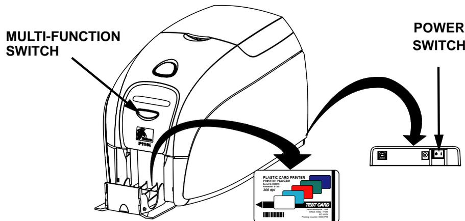
3. Keep pressing the Multi Function button until the SELF TEST message appears in the window.
