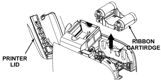
2. Open the lid and remove the ribbon cartridge.
