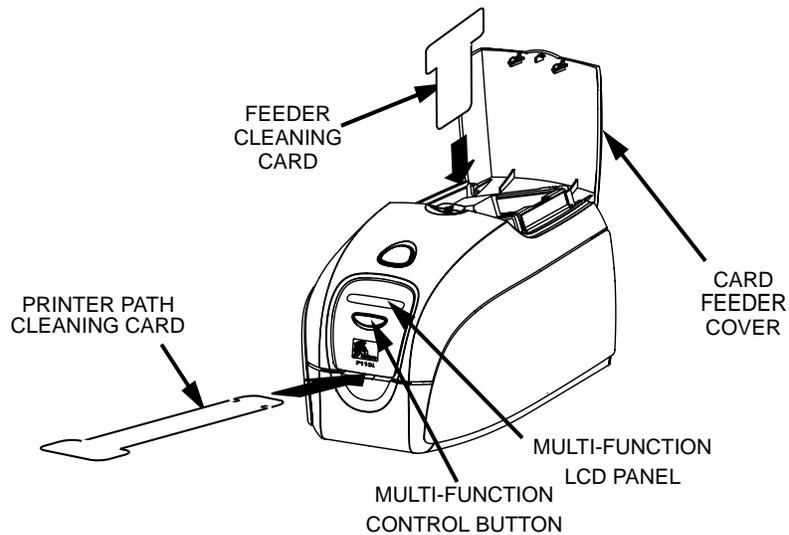
4. After the ribbon is removed and the lid is closed, the message **EMPTY FEEDER THEN CLOSE COVER** will display.
