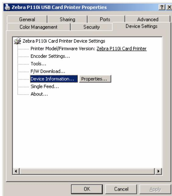
9. On the Device Settings tab, you can change settings for a Magnetic Encoder and change to or from single feed mode.
