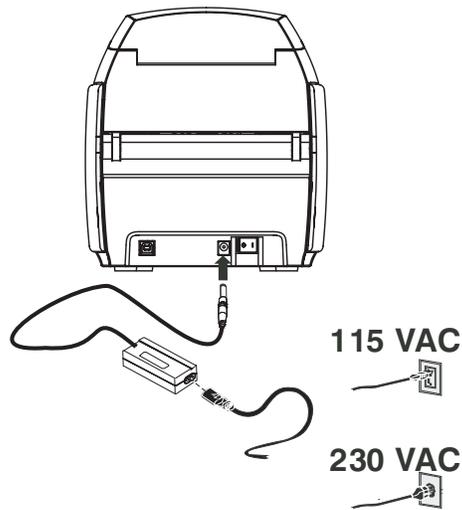
4. Insert the power supply plug into the power socket, attach the power cord (120VAC or 230VAC) to the power supply, then plug the power cord in to a grounded electrical socket of the proper voltage and type.
