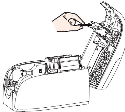
3. Clean Print Head by moving alcohol-moistened swab tip side-to-side across Print Head elements. Only use moderate force.
