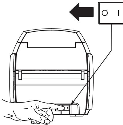
3. Ensure that the printer's power switch in the OFF ( O ) position.
