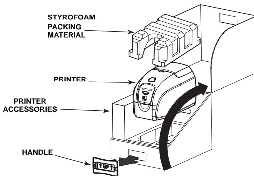
4. Lift the printer out of the carton by holding it on both sides of the bottom and lifting the printer gently from the carton.
