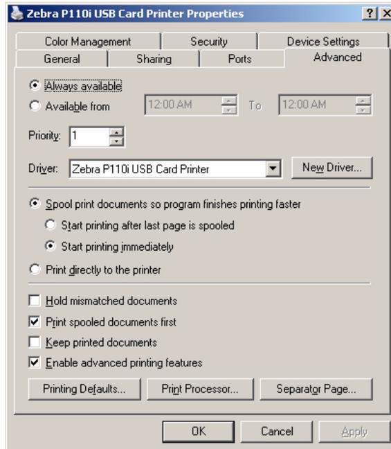
8. On the Advanced tab, you can choose various printer properties, install different printer drivers, and change default printer settings.
