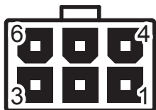
POWER SUPPLY Male Molex connector vertical (no. 39-30-0060)
