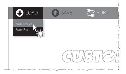
Click on LOAD > FROM DEVICE and select the device connected to the PC.
