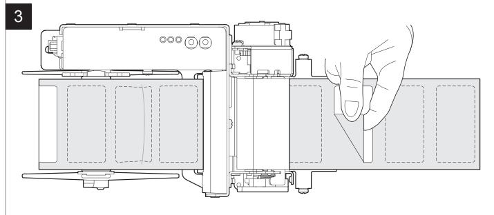
Remove all labels on the support near the paper inlet and bezel.
