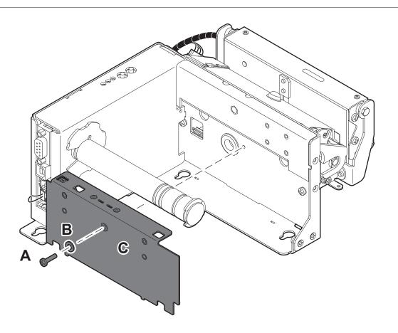
Unscrew the fixing screw A and remove the washer B. Move the lower paper guide away C being careful not to damage the cables.
