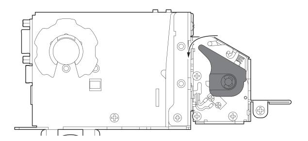
Close the printhead by rotating the printhead lifting lever.
