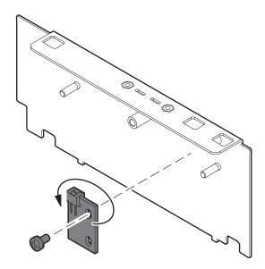
To position the sensor in position B, rotate the sensor 180 ° and fix it in the previous position with the previously removed fixing screw.
