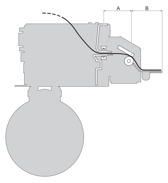
A = distance between printhead and alignment sensor = 36.5 mm B = distance between printhead and peeler output = 47 mm
