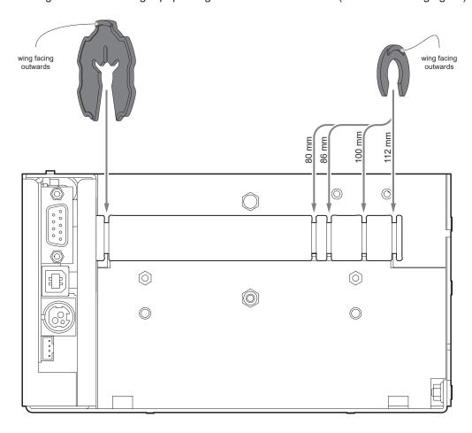
To manage paper width of 80, 86 or 100 mm, fix and correctly place the paper guide bracket provided with the device. The following figure shows an example of bracket fixing for 80 mm paper width.
