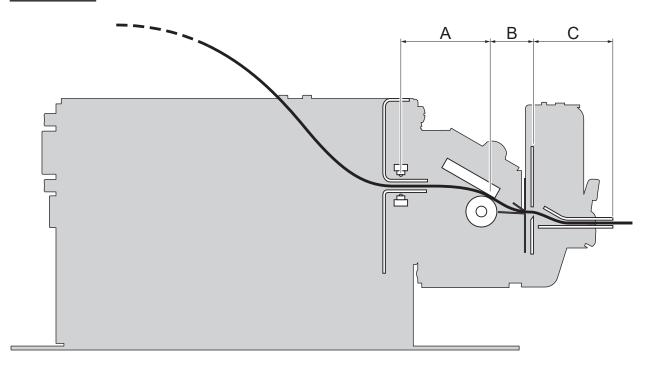
A = distance between printhead and alignment sensor = 34 mm
