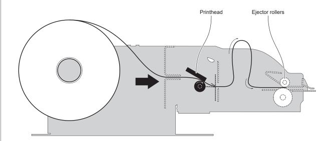
The ticket advances ahead to the ejector and is caught between the ejector rollers. The printed part of ticket is collected into the ejector group while the device continues printing.
