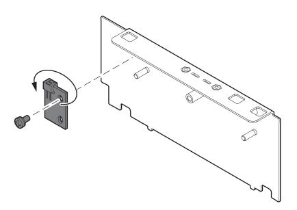
To position the sensor in position C, rotate the sensor 180 ° and fix it in the position indicated with the previously removed fixing screw.
