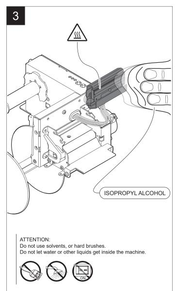
Clean the printhead by using a non-abrasive cloth moistened with isopropyl.
