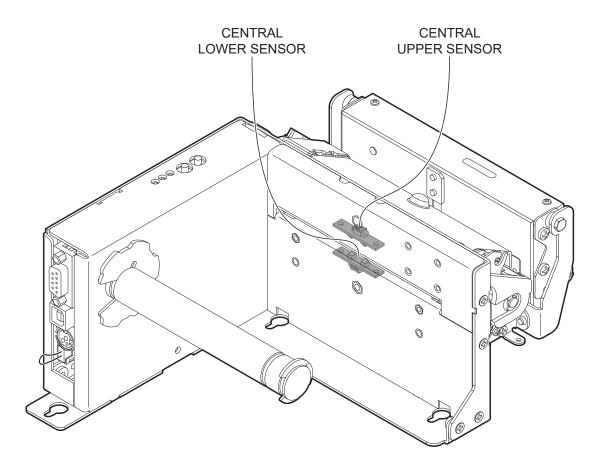
To guarantee the correct alignment, you must enable the parameter "Black Mark Position" during the setup procedure (see chapter 6).
