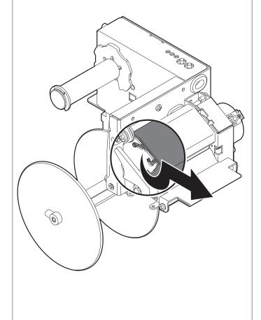
Unlock the printing mechanism as shown in figure.
