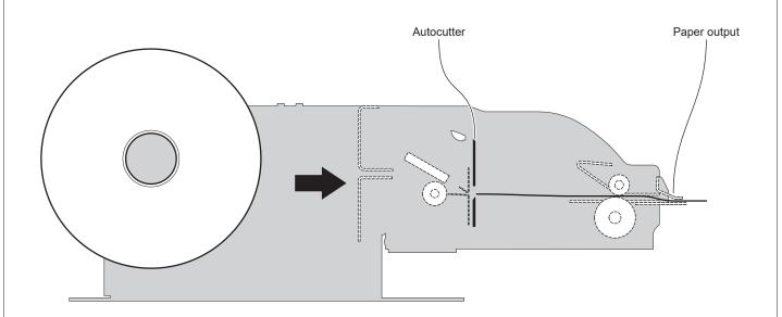
When printing ends, the device cuts the ticket printed.
