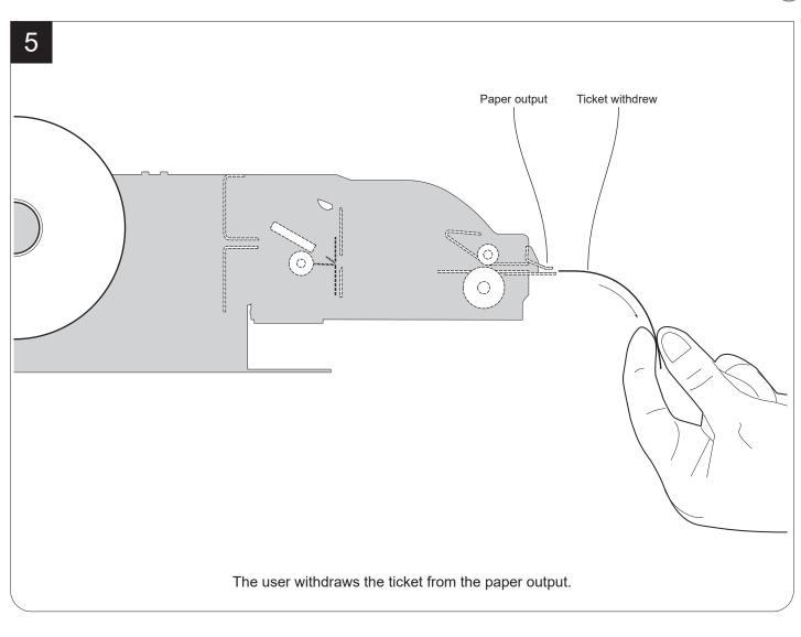
NOTE: To enable this issuing mode, you need to correctly set the operation mode of the ejector with the command 0x1D 0x65 (see commands manual) and the setup parameter "Automatic Ejecting" (see chapter 6).
