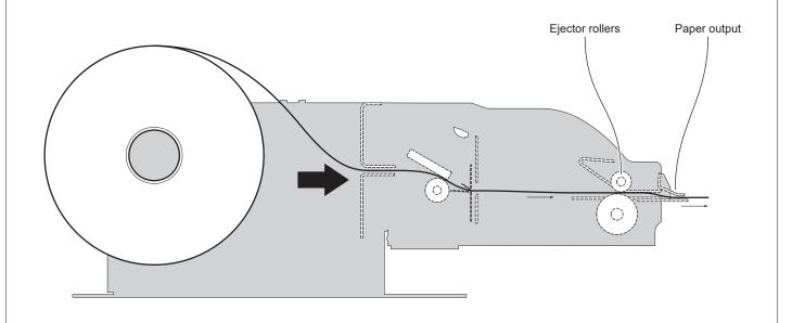
The ticket goes beyond the ejector rollers and stanrts to come out of the paper output.
