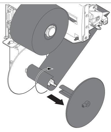
Remove the rewinder plastic disk and wrap the paper around the pin as indicated by the arrow.
