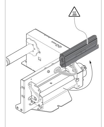
Unlock the printing mechanism by following the specific procedure for each model as described in the previous paragraphs.
