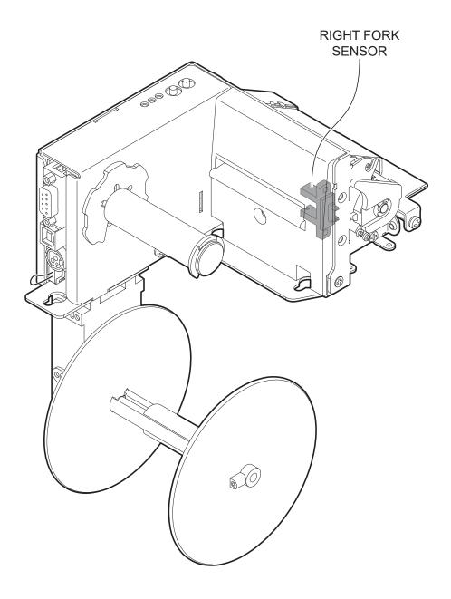
To guarantee the correct alignment, you must enable the parameter "Black Mark Position" during the setup procedure (see chapter 6).
