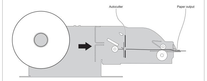
When printing ends, the device cuts the ticket printed.
