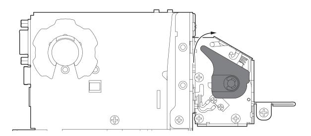
Open the printhead by rotating the printhead lifting lever.
