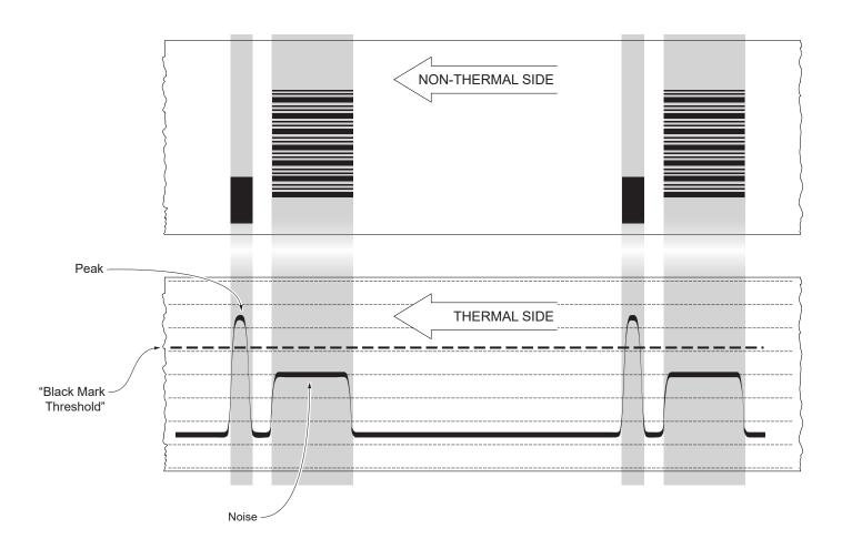
If the maximum value of "noise" read by the sensor is very close to the peak value, it might be difficult to place the value of the "Black Mark Threshold" at an intermediate point. In these cases, it is mandatory that the portion of paper between the point of printing end and the front notch is completely white (no graphics). In this way, the only next graphic detected by the sensor for alignment after the printing end will be the notch.
