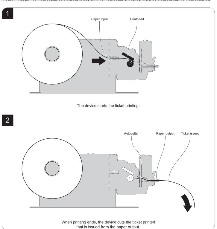
NOTE: To enable this operating mode, you need to send a cut command when the printing ends (see commands manual).
