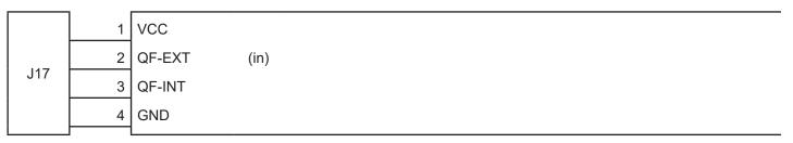
The following figure shows the pinout of the connector of the cable for low paper to use for the device:
