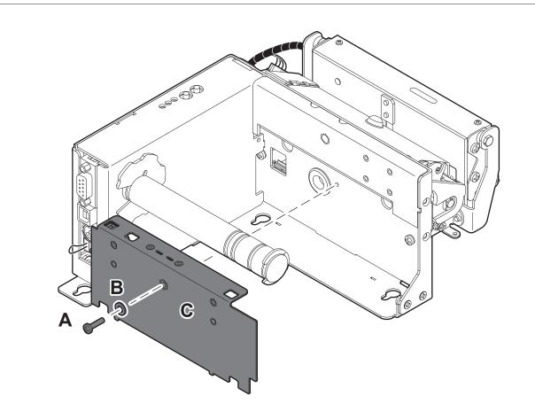
Reposition the lower paper guide C in its seat and fix it with the fixing screw A and the washer B.
