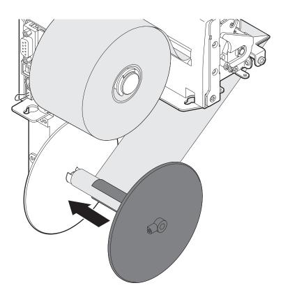
Block the paper by inserting the plastic disk.
