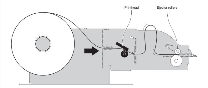
The ticket advances ahead to the ejector and is caught between the ejector rollers.
