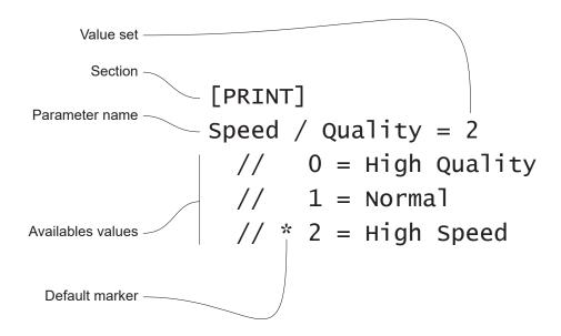
To modify the parameter, change the numeric value after the parameter name or use the default value by typing "D". After editing device's parameter, simply save the "Setup.ini" file to make the modifies activated. For a detailed description of the device operating parameters see the following paragraphs.
