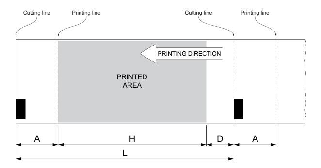
A "Non-printable area" = "Distance between autocutter/printhead"
