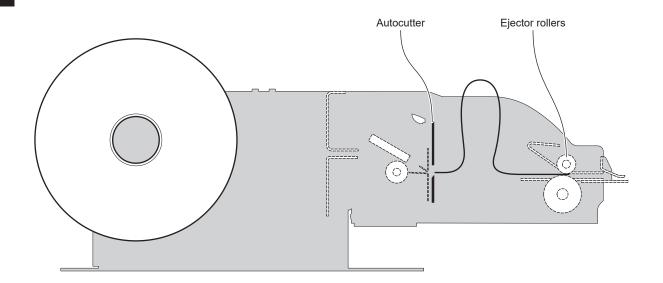
When printing ends, the device cuts the ticket printed
