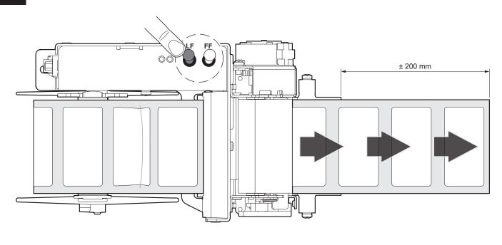
Press the LF LINE FEED button repeatedly to advance the paper of at least 200 mm beyond the edge of the peeler.
