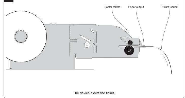
NOTE: To enable this issuing mode, you need to correctly set the operation mode of the ejector with the command 0x1D 0x65 (see commands manual) and the setup parameter "Automatic Ejecting" (see chapter 6).
