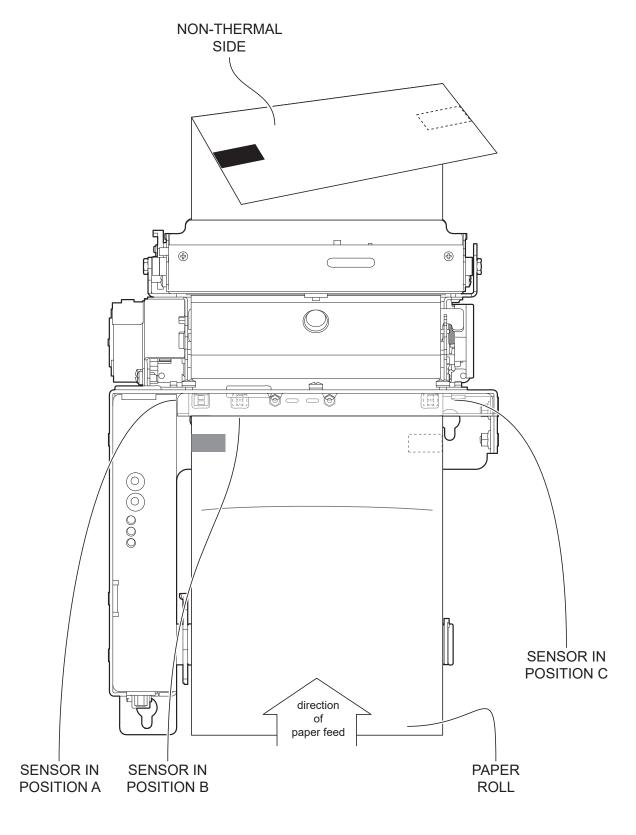
To guarantee the correct alignment, you must enable the parameter "Black Mark Position" during the setup procedure (see chapter 6).
