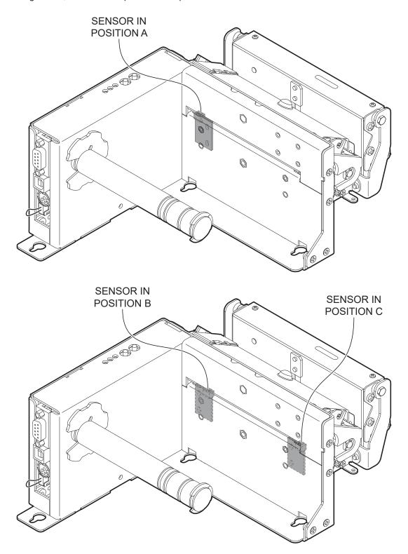
To place the sensor in positions B or C, proceed as follows.
