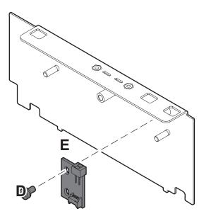
Unscrew the fixing screw D and remove the alignment sensor E.
