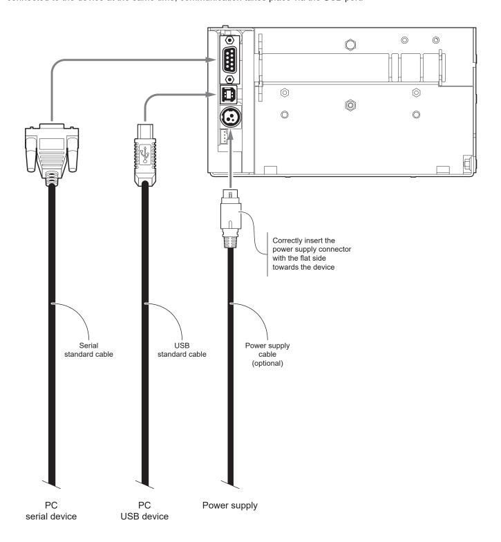
ATTENTION: In some conditions, we recommend the installation of a ferrite core on the power supply cable.
