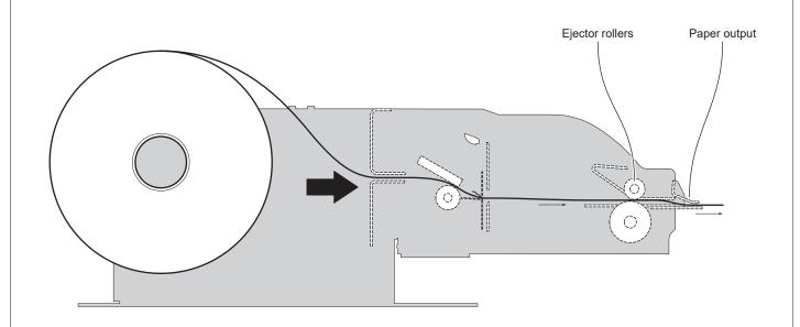
The ticket goes beyond the ejector rollers and starts to come out of the paper output.
