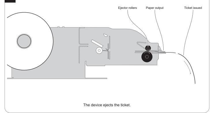
NOTE: To enable this issuing mode, you need to correctly set the operation mode of the ejector with the command 0x1D 0x65 (see commands manual) and the setup parameter "Automatic Ejecting" (see chapter 6).
