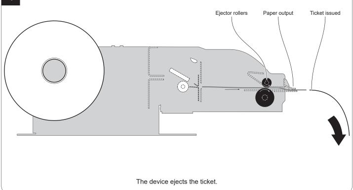
NOTE: To enable this issuing mode, you need to correctly set the operation mode of the ejector with the command  $0x1D\ 0x65$  (see commands manual).
