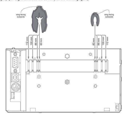
To manage paper width of 80, 86 or 100 mm, fix and correctly place the two paper guide brackets provided with the device. The following figure shows an example of bracket fixing for 86 mm paper width.
