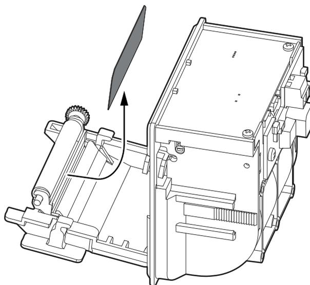
Remove the anti-jam separator by detaching it from the cover.
