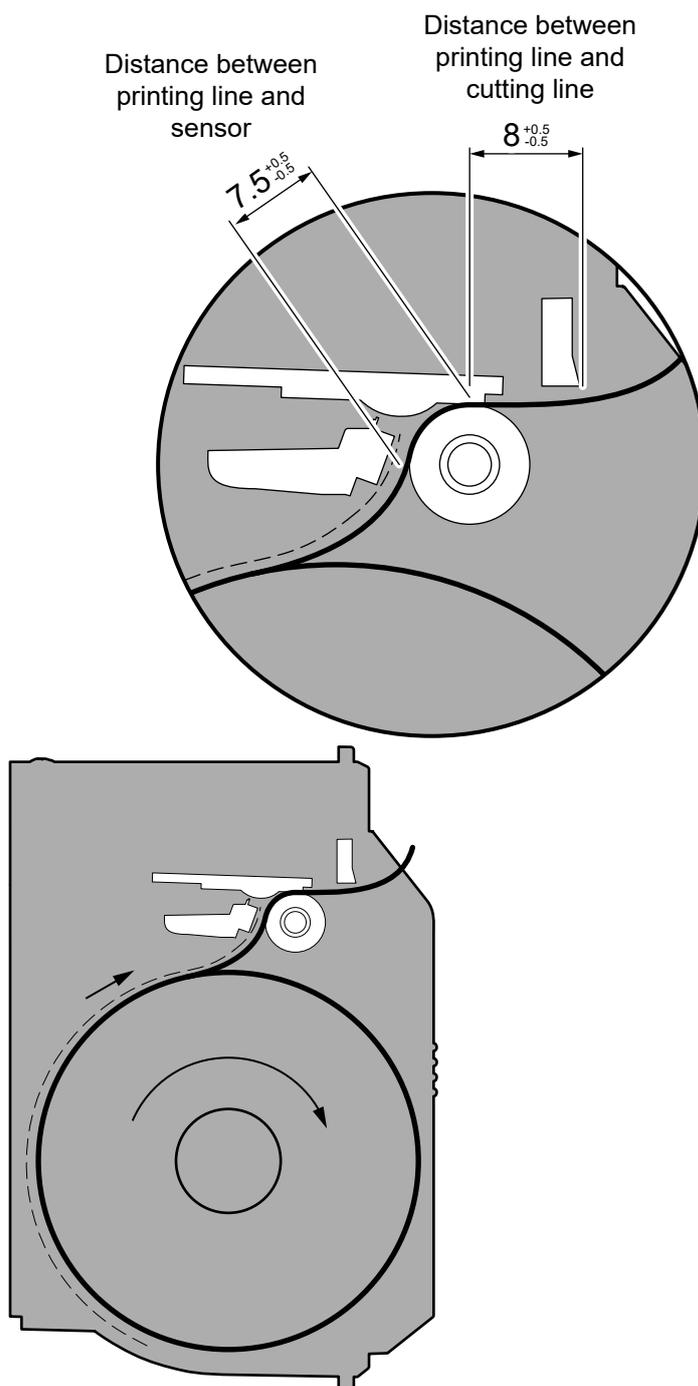
To define the alignment point you need to set the printer parameters that compose the numerical value of the “Black Mark Distance” parameter (see [paragraph 5.6](#)).
