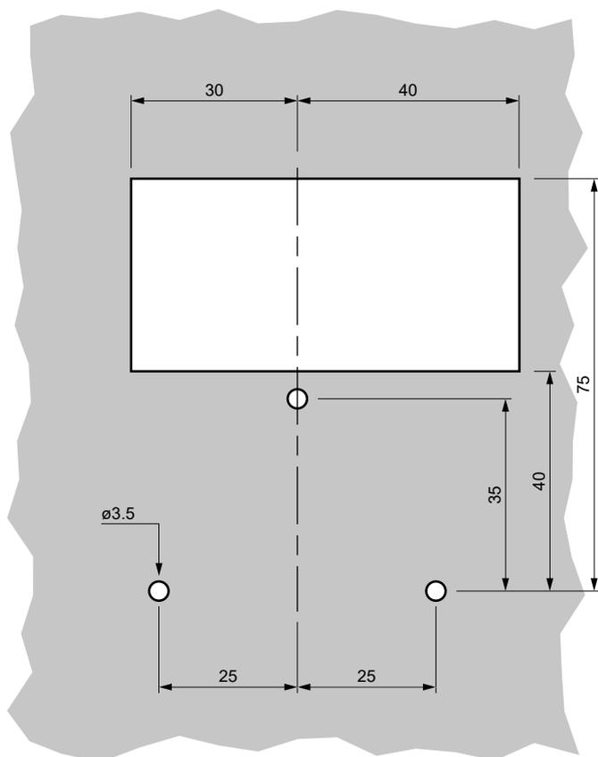
Drilling for mounting on panel with
