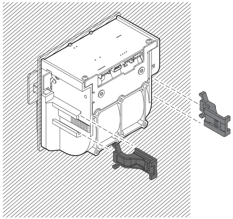
Insert the fixing clips into the seat on both the device sides.
