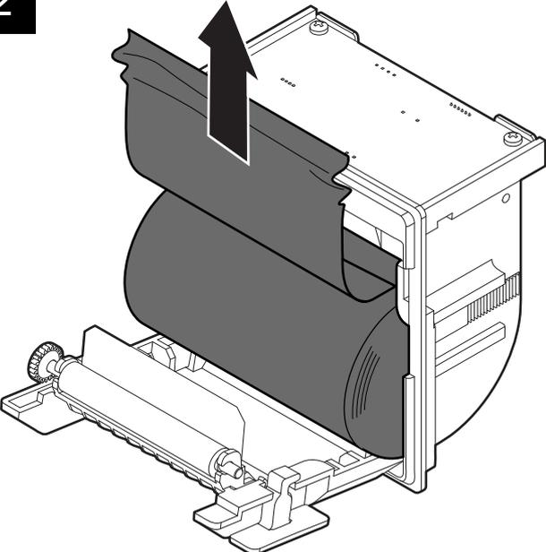
Lift the damaged paper, check and remove any scraps of paper. Pull the paper so that the damaged part remains outside the device.
