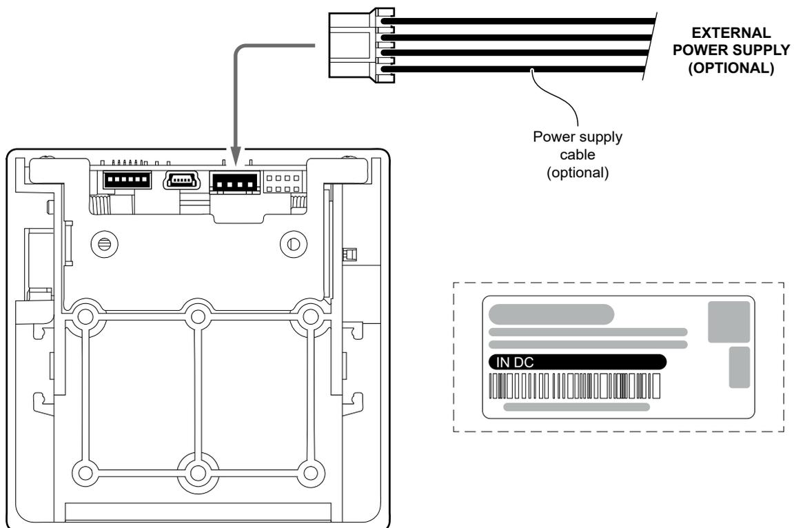
Connect the power supply cable to an external power supply unit and to the device.
