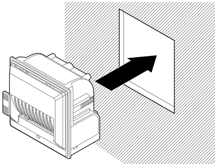
When the device is installed in the upside down position, pay attention when opening the paper compartment cover (see [paragraph 4.1](#)) to prevent the paper roll from falling and unrolling.
