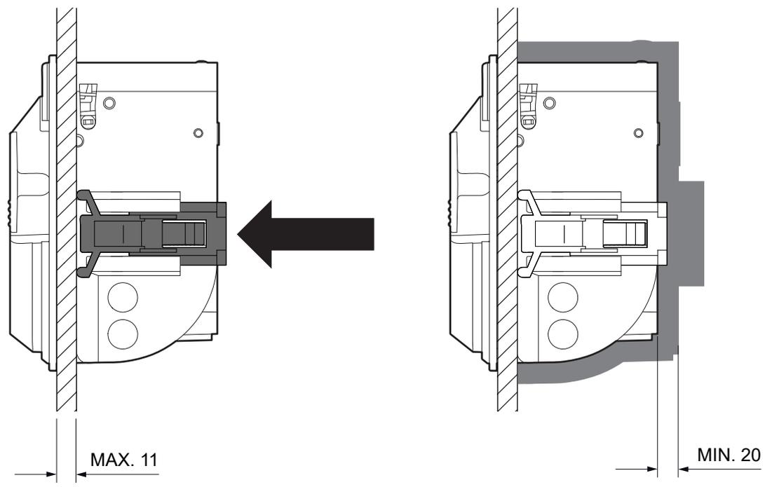
Push the two fixing hooks to strike the panel.
