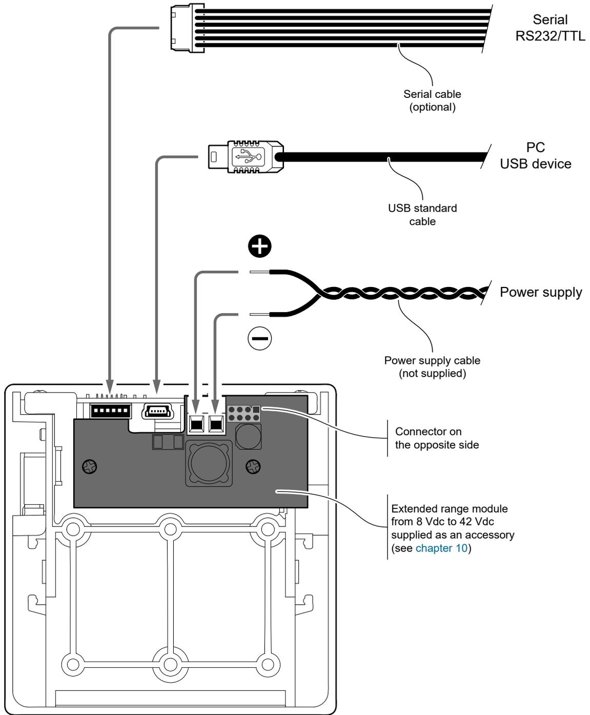
**ATTENTION:** In some conditions, we recommend the installation of a ferrite core on the power supply cable.
