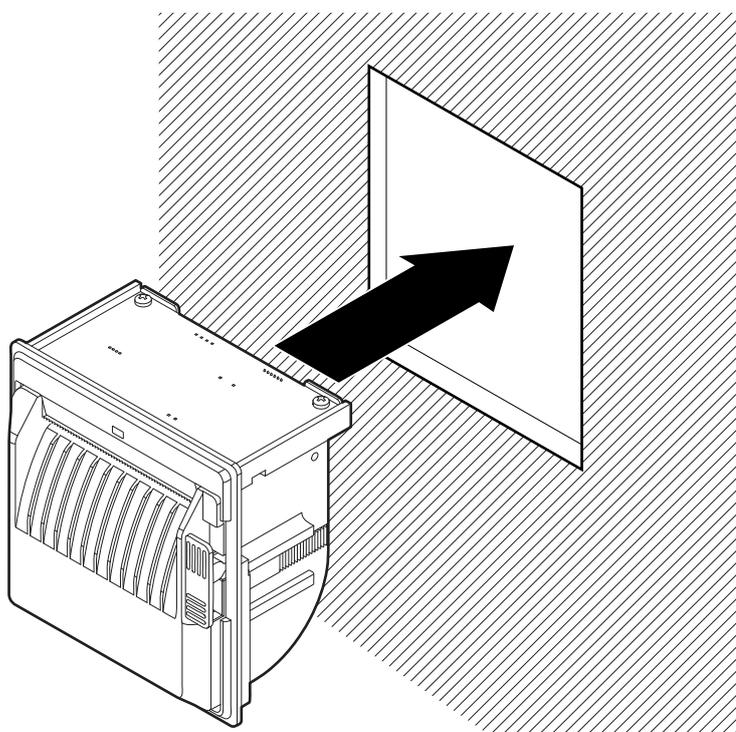
Insert the device inside the panel.
