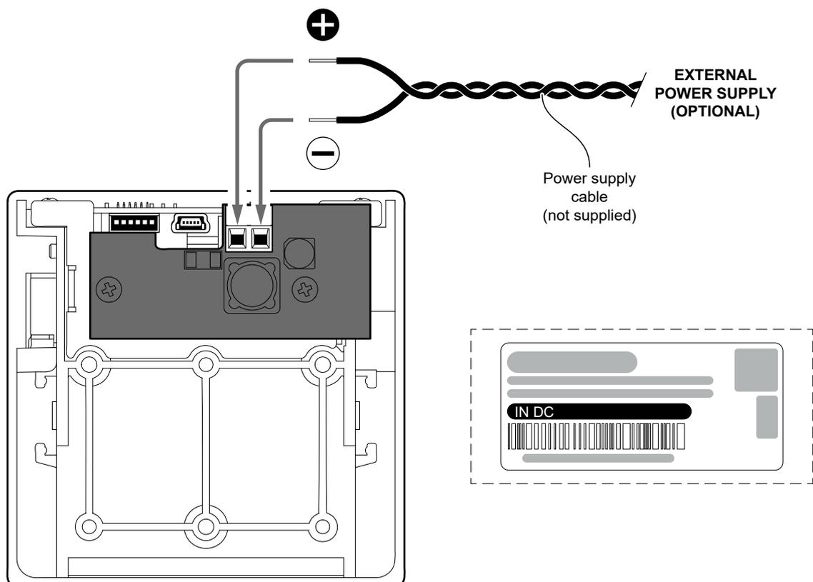
Connect the power supply cable to an external power supply unit and to the device.
