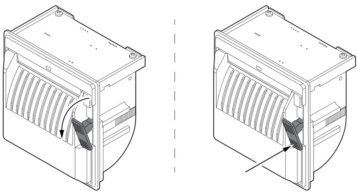
Wide the upper portion or push on the lower portion of the opening lever to unhook the cover of the paper compartment.
