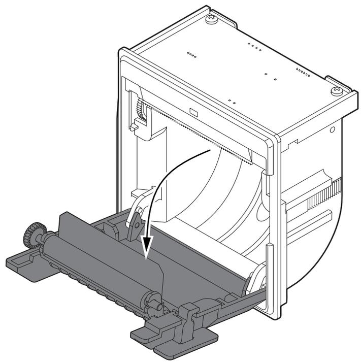
Open the cover of the paper compartment completely.
