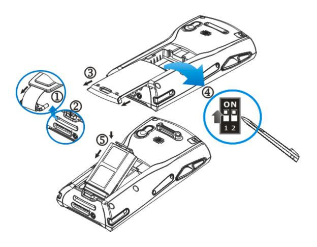
Figure 5: Installing the Main Battery
