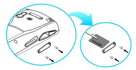
Figure 3: Inserting the miniSD Card
