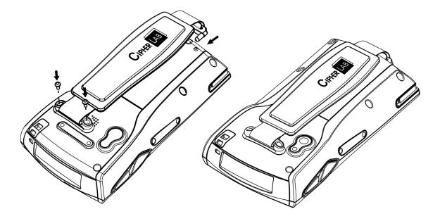
Figure 2: Installing the Hand Strap
