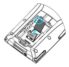
Figure 4: Inserting the SIM Card
