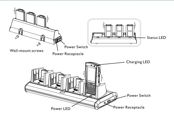
Figure 9: 4-Slot Battery Charger (top); 4-Slot Charging Cradle (bottom)
