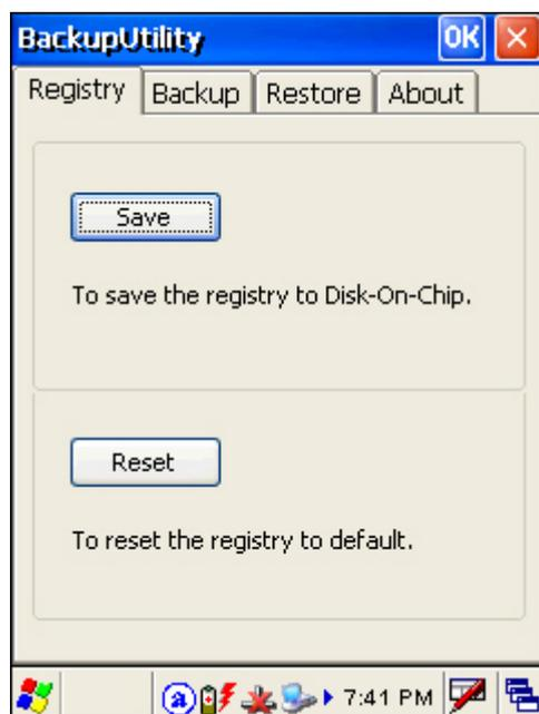
**Warning:** As long as you make any changes to the system configurations and settings, you must tap [Save] to update the system registry here. Otherwise, it will reload the old registry values in use after a cold boot.
