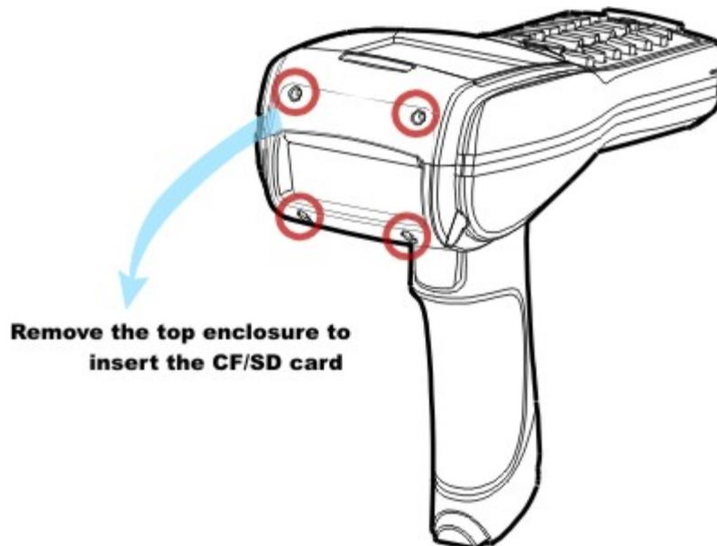
*Figure 4: Inserting the SD or CF Card*
