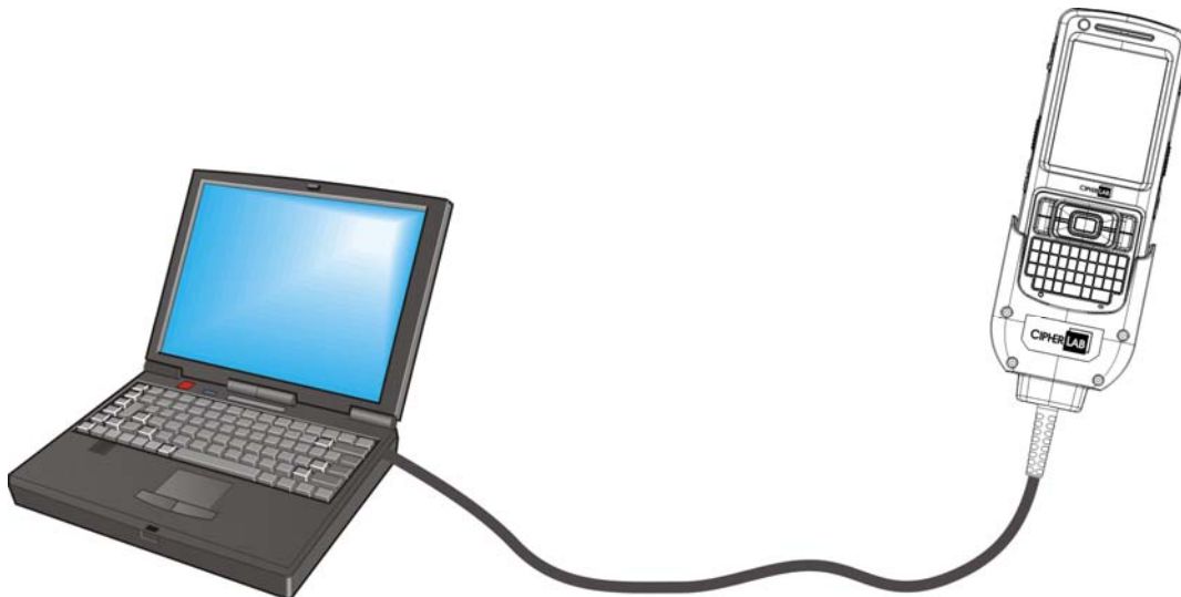
Figure 11: Direct Data Communication Using Snap-on Cable
