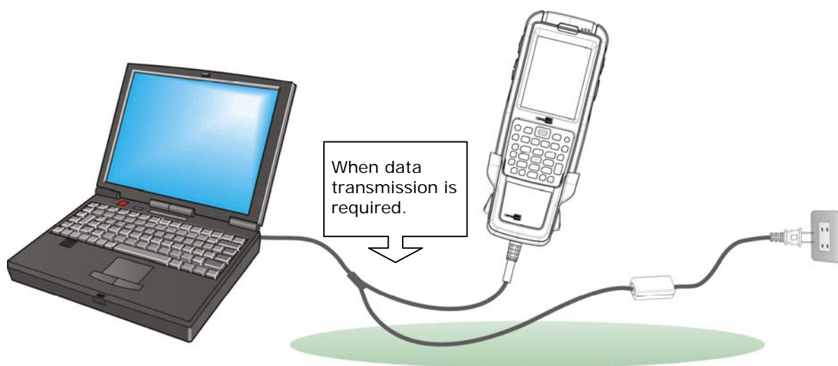
Figure 5: Direct Charging Using Snap-on Cable
