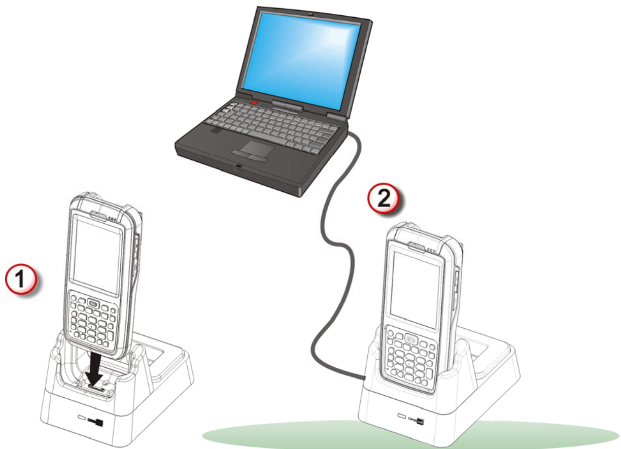
Figure 12: Direct Data Communication Using Cradle
