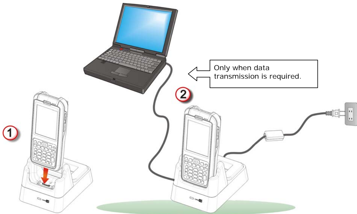
Figure 6: Direct Charging Using Cradle
