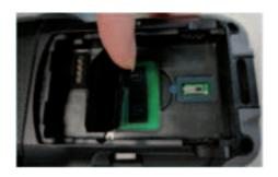
• As the diagram shown, insert SIM Card and MicroSD.
