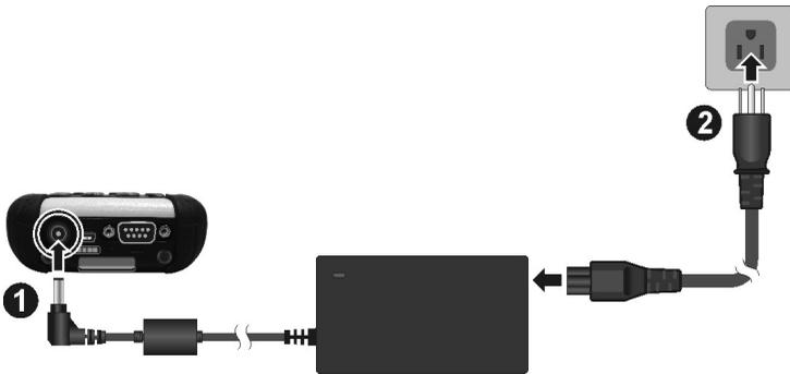
3. The charge indicator glows in amber when charging is in progress. Do not disconnect your device from AC power until the battery is fully charged, as indicated by the amber indicator turning into green. This will take a couple of hours.
