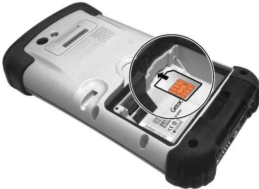
**NOTE:** To remove the SIM card, slightly push in the card to release it and then pull the card out of the slot.
