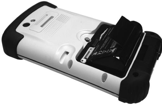
4. Attach the bottom side of the battery cover to the device at an angle and then, with the handle still in the unlock (vertical) position, fit the latch handle into place. Secure the latch by turning it clockwise to the lock (horizontal) position.
