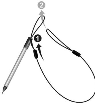
2. Insert the other loop end to the holder on the device (as indicated by ❶ below). Then, insert the stylus end through the loop (as indicated by ❷ below) and pull it tight.
