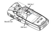
4. Replace the battery and the cover. Slide the cover latch to the lock position.
