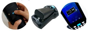
Easily change the HT730 battery without interruption / rebooting the device. Reboot within 1 minute - screen will automatically start the countdown.
