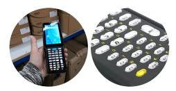
Keypad with backlight design. Durable keypad with 2.5 million lifetime clicks. Hard silicon material with key printing underneath keys.
