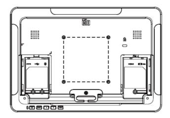
For the 15-inch touchmonitor, a four-hole 75x75mm and 100x100mm mounting pattern for M4 screws is provided on the rear of the monitor. Remove the stand using a Phillips screwdriver to access this mounting interface. The VESA FDMI-compliant counting is coded: VESA MIS-B, 75, C and VESA MIS-B, 100, C.
