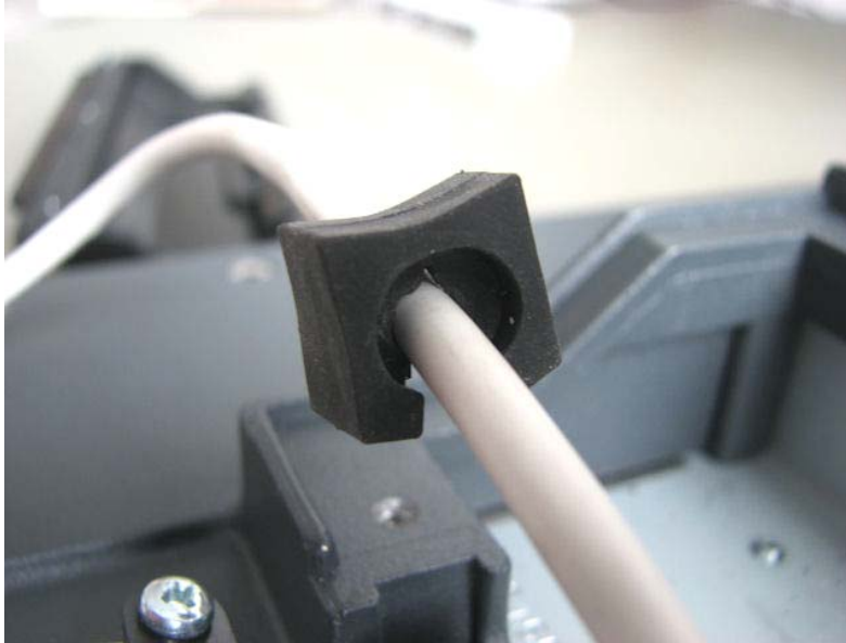
Figure 7.5: Sleeve around a cable
