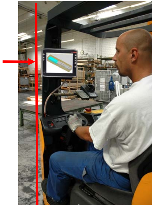
Figure 7.2: Position of the MTC 6 on a forklift
