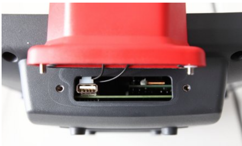
Figure 7.4: Opened antenna cap
