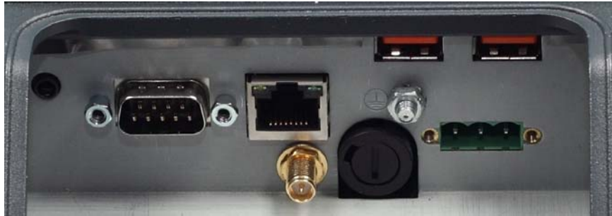
Figure 5.7: External connectors with optional ext. antenna
