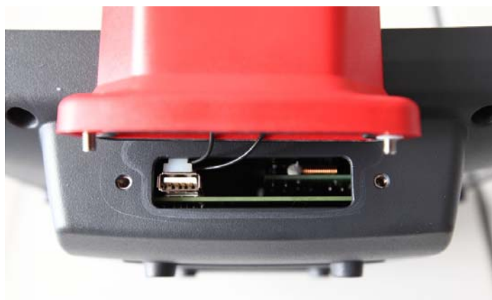
Figure 5.11: Service USB under the antenna cap
