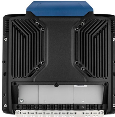
Fig. 13.1: VESA mounting hole pattern on the rear side of the DLT-V73
