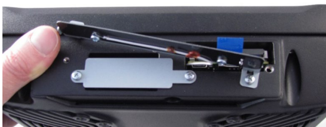
Fig. 15-4: opened WLAN Diversity Antenna
