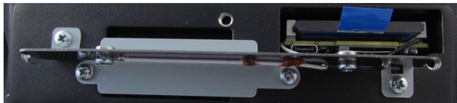
Fig. 7.7: WLAN antenna cap IEEE 802.11 a/b/g/n/ac/ax opened
