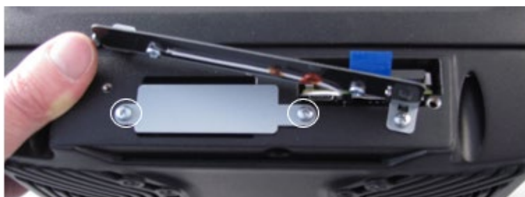
Fig. 15-5: Screws from the battery cover
