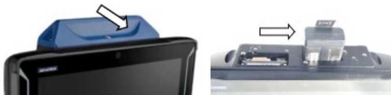
Fig. 15.1: Battery pocket with UPS DLT-V73
