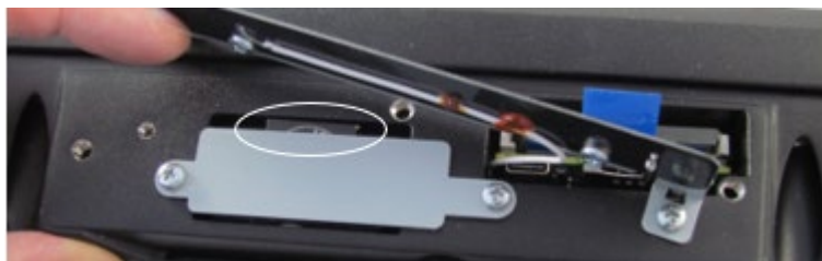
Fig. 15-8: Removal tab under the battery cover
