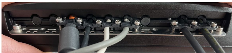
Fig. 14.14: Cable cover closed and screwed together
