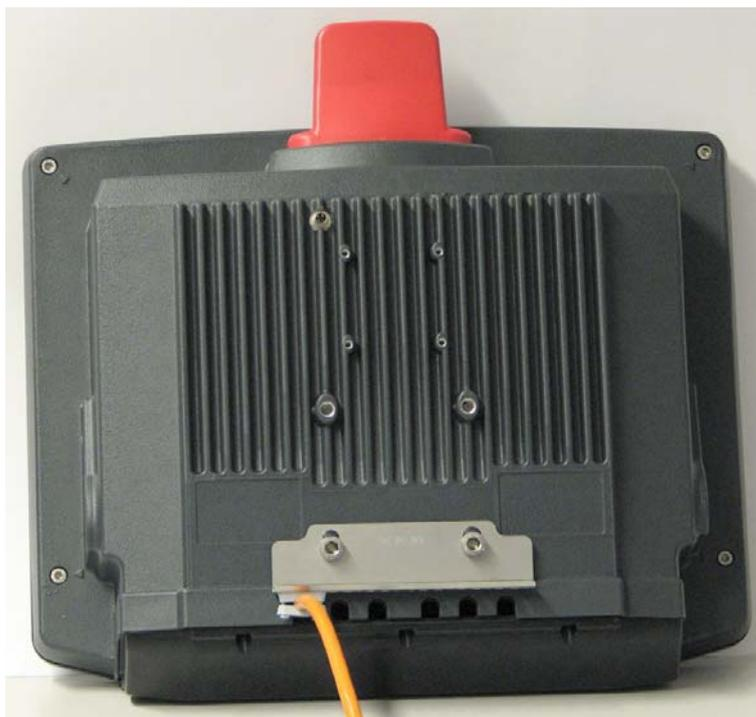
Figure 7.8: DLoG IPC 7/215 with cable cover mounted
