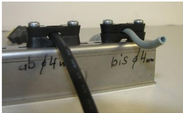
Figure 7.4: Strain relief clamps
