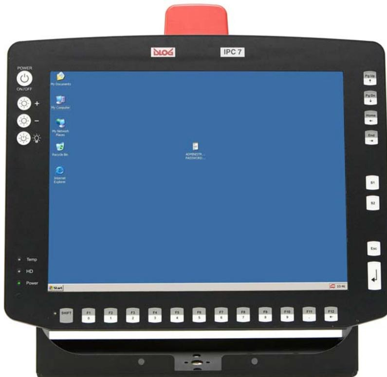
Figure 8.2: DLoG IPC 7/215 front panel with 25 keys
