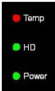
Temp (red) LED indicates an excessively high or low temperature inside the unit
