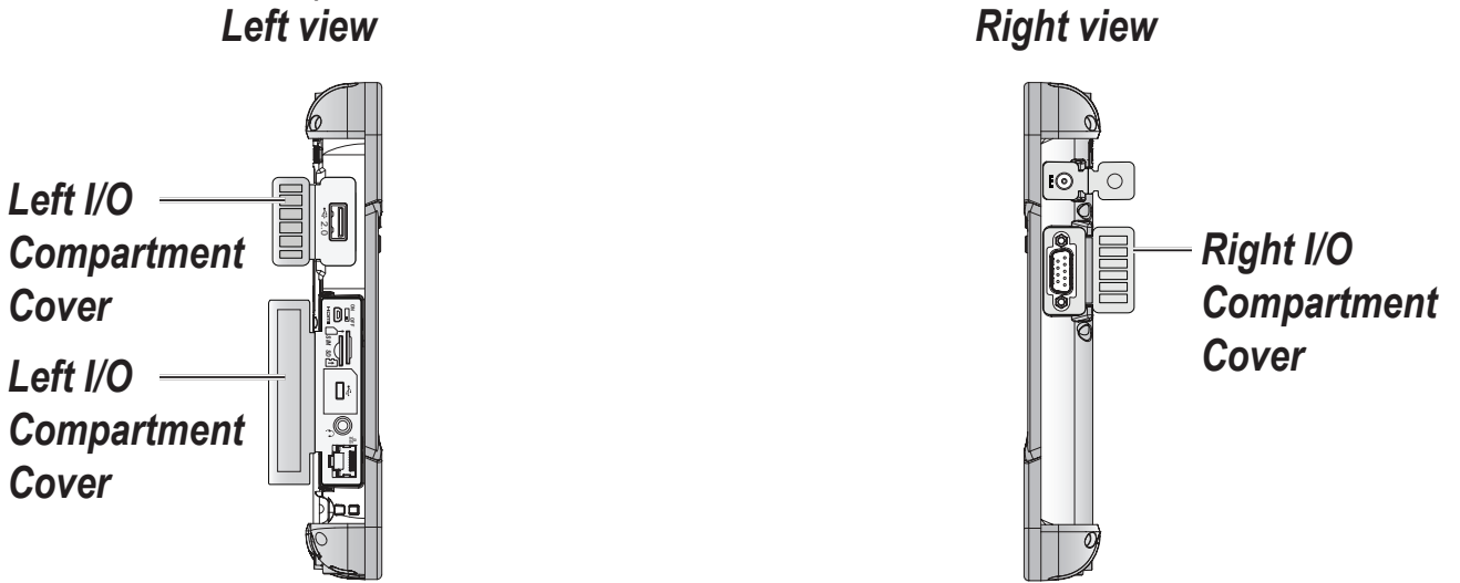
Figure 26. Side View: Locating the I/O Compartment Cover
