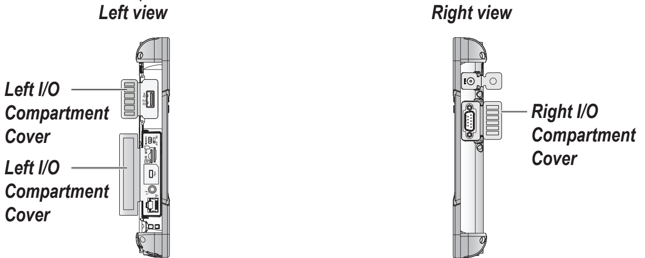
Figure 23. Side View: Locating the I/O Compartment Cover
