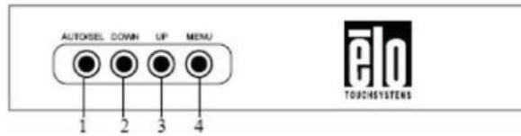
The On-Screen Display (OSD) Remote Control Box is an optional accessory that allows you to change settings on the monitor screen remotely. It has four buttons:
