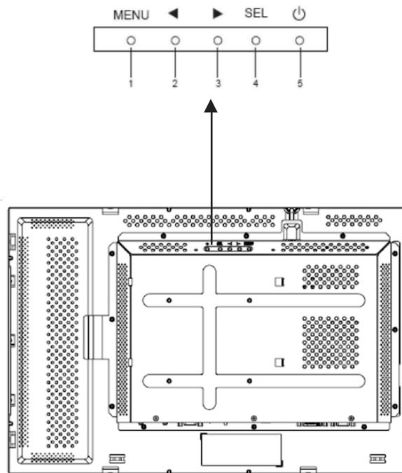
The rear panel control buttons for on-screen display (OSD) adjustments allow you to change settings on the monitor screen. There are five buttons:
