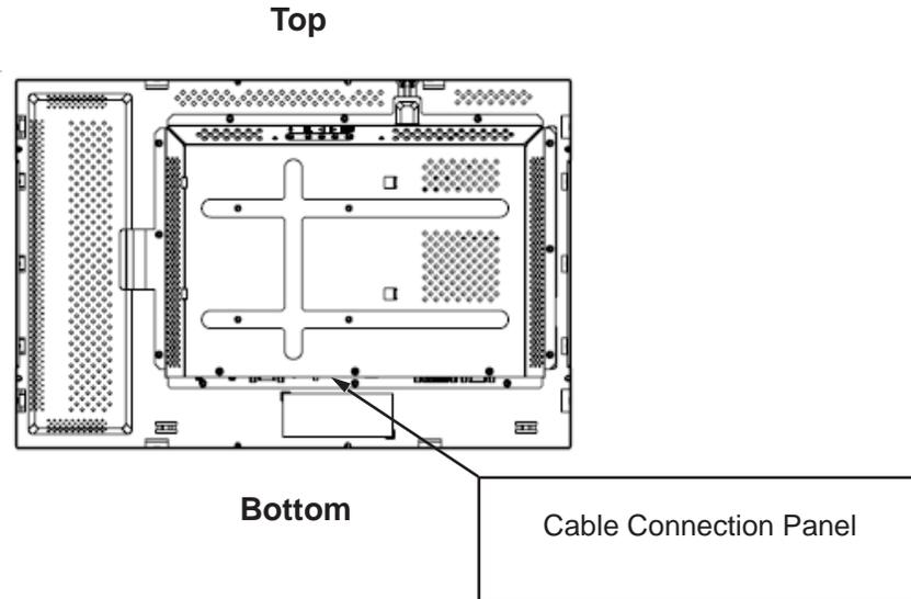
Alternatively, the monitor may be mounted in the portrait orientation. For this orientation, the cable connection panel may be on either side, as shown in the illustrations below.
